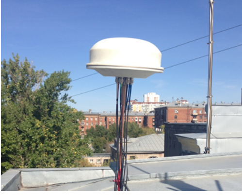
Figure 4: Seven-element L1-band convex antenna based on a university building roof
